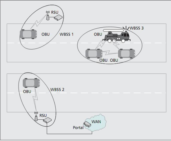
Fig. 1. Illustration of a WAVE system showing the typical locations of the onboard units (*OBUs*) and roadside units (*RSUs*), the general makeup of the WBSs, and the way a WBS (WAVE Basic Service Set) can connect to a WAN through a *portal*.
