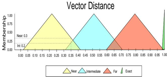
Fig. 3. Fuzzy Input Membership Function for the Vector Distance Factor and a Sample Fuzzification
