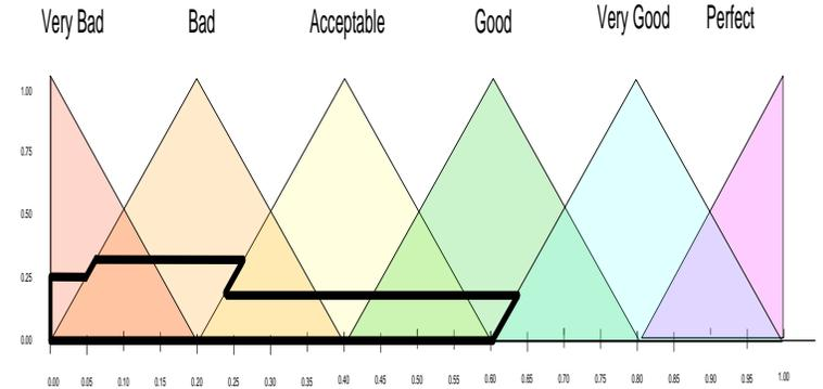
Fig. 7. Output Membership function and an example of the resulting shape of function  $f(x)$
