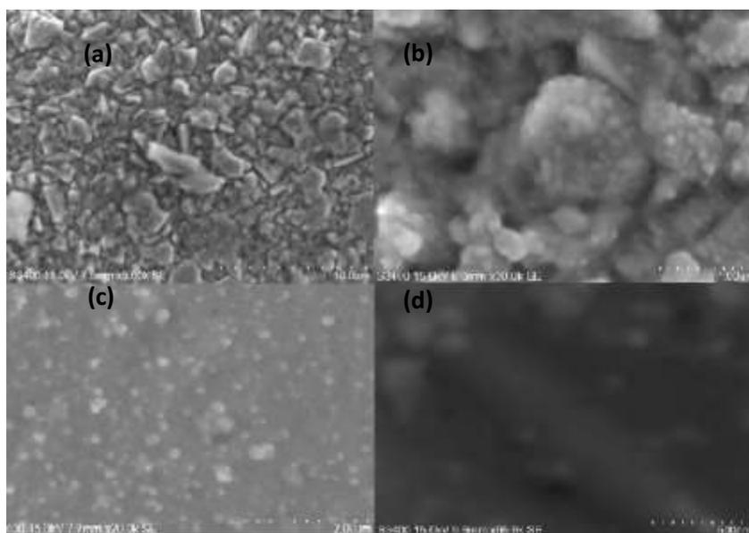
**Figure 5.** SEM images from (a) 2:1 TiO<sub>2</sub>:PAA with 5,000x magnification, (b) 1:1 TiO<sub>2</sub>:PAA and (c) 1:2 TiO<sub>2</sub>:PAA with 20,000x magnification and (d) 2:1 TiO<sub>2</sub>:PAA with 85,000x magnification in Copper TEM grids
