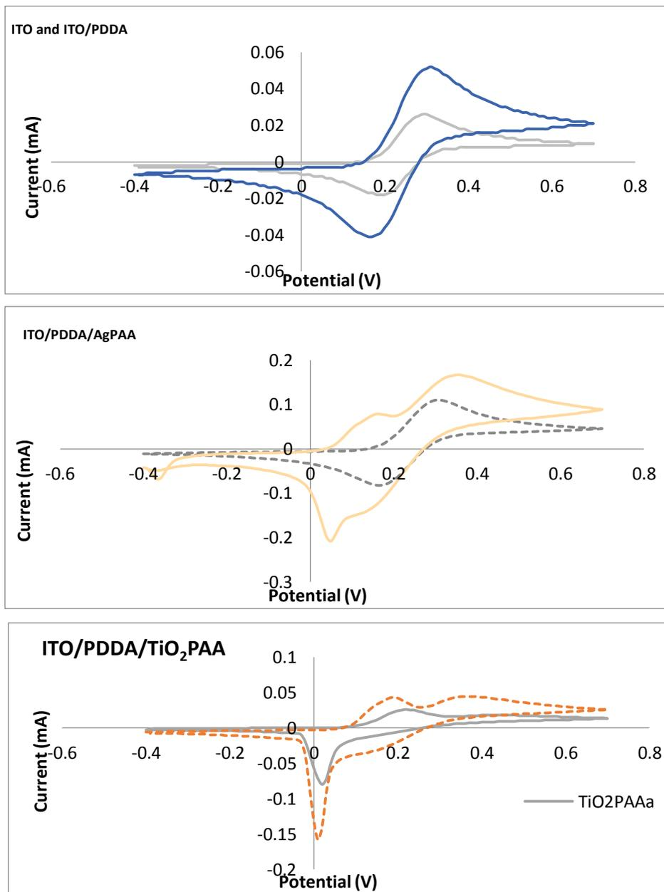
Figure 11: (*Top*) Reversible CV of bare ITO and PDDA on ITO taken on the 3<sup>rd</sup> cycle. (*Middle*) CV of 5 layers PDDA/Ag/PAA on ITO (dashed = 1<sup>st</sup> cycle, line = 2<sup>nd</sup> cycle). (*Bottom*) CV of 5 layers PDDA/TiO<sub>2</sub>PAA on ITO (a = 1<sup>st</sup> cycle, b = 2<sup>nd</sup> cycle)
