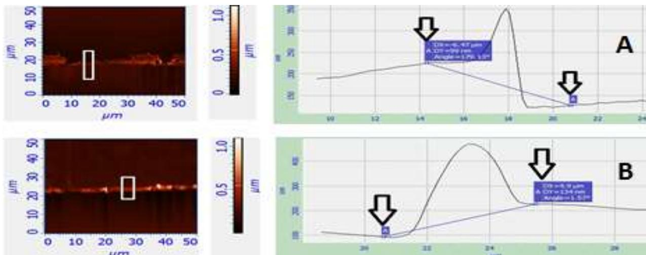
Figure 9. Images of 50  $\mu\text{m}$  x 50  $\mu\text{m}$  scan size of scratched surface of 25 layers PDDA/Ag/PAA on glass slide (A) and quartz slide (B) with corresponding AFM average cross sectional plot. Film thicknesses (DY) were 99 nm (A) and 134 nm (B)
