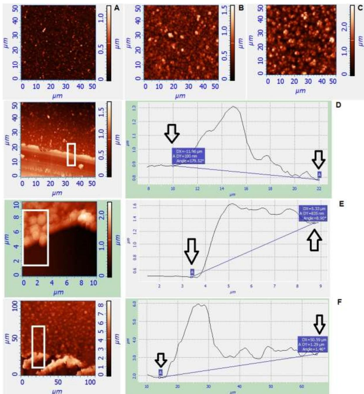
Figure 10. Surface images before scratching the surface of  $(\text{PDDA}:\text{TiO}_2\text{PAA})_n$  on glass slide (450 kDa PAA):  $n = 5$  (A), 10 (B) and 15 (C). Height profiles for 5 (D), 10 (E) and 15 (F) layers after scratching the surface.
