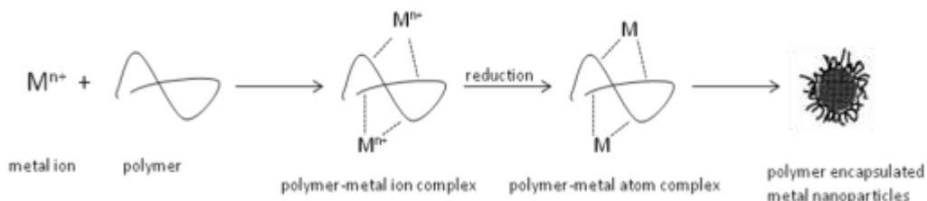
Figure 1. Schematic illustration of the process for the polymer protected metal nanoparticles.
