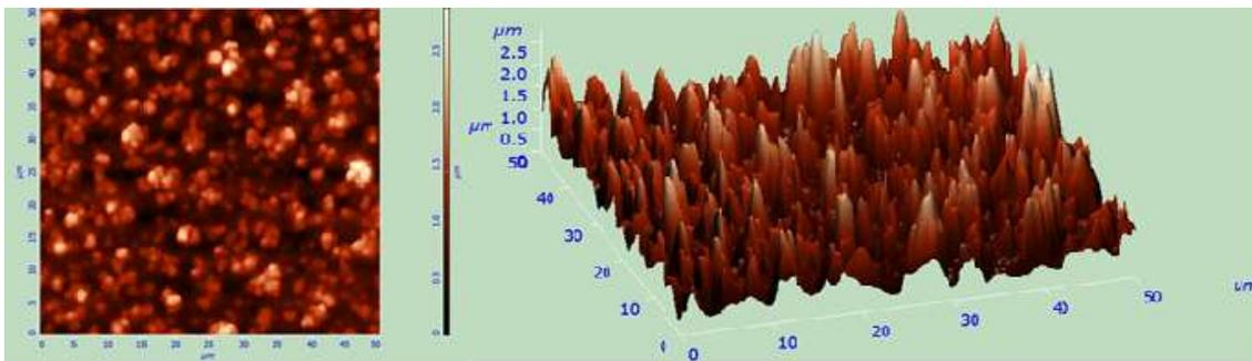
**Figure 8.** Images of the film formed by LbL deposition of 1:2 TiO<sub>2</sub>:PAA solution with PDDA in an area of 50 x 50 μm<sup>2</sup> generated by AFM imaging (left) 2D and (right) 3D for (a) 5 layers, (b) 10 layers and (c) 15 layers
