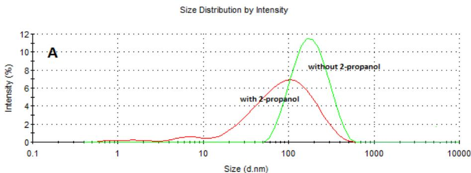
Figure 4. Dynamic Light Scattering Histogram of Ag/PAA (with and without 2-propanol)
