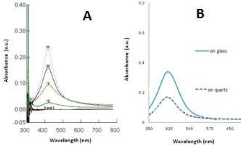
Figure 6. A. Surface plasmon band of  $(\text{PDDA:Ag/PAA})_n$  multilayer film where  $n$  is the number of layers (5, 10, 15, 20, and 25); (B) plasmon bands for 25 layers of Ag/PAA/PDDA on glass slide (indicated as line) and quartz slide (dash).
