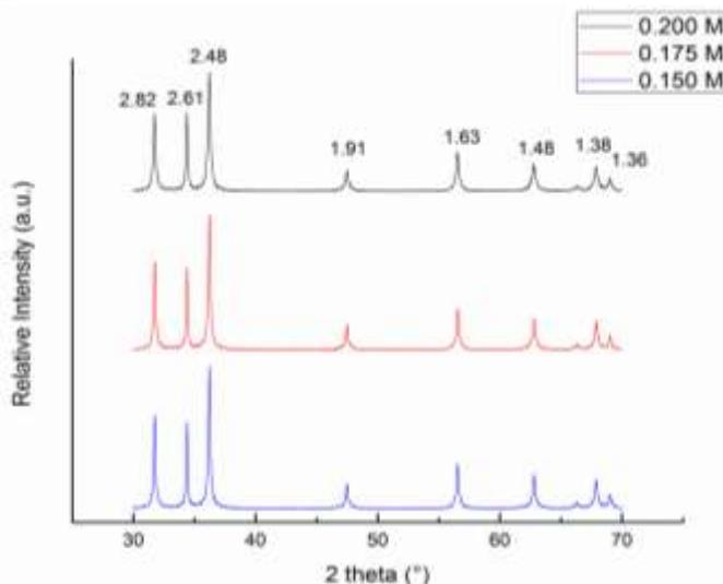
Figure 1: XRD pattern of produced ZnO for different molarities
