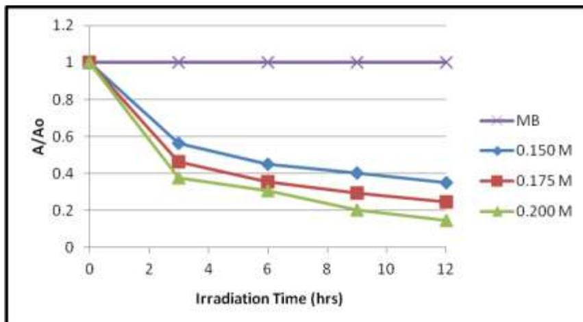
Figure 4: Extent of degradation of Methylene Blue (A/A<sub>0</sub>) as a function of irradiation time
