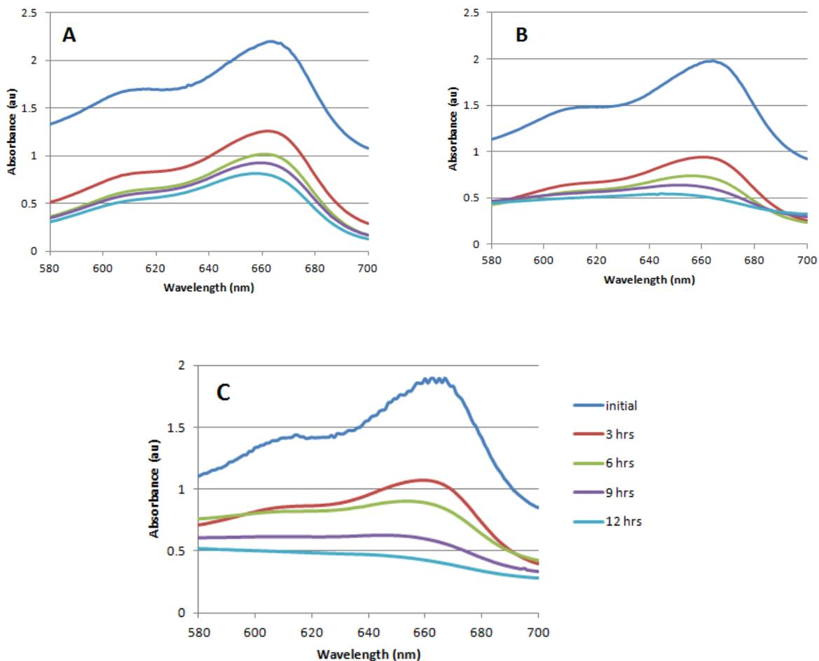
Figure 3: Absorbance for varying UV exposure time for different precursor molarities: (A) 0.150 M, (B) 0.175 M. (C) 0.200 M
