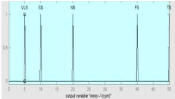
Figure 6: Membership function for motor 1 (rpm)
