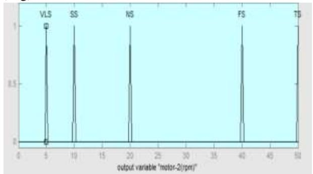
Figure 7: Membership function for motor 2 (rpm)
