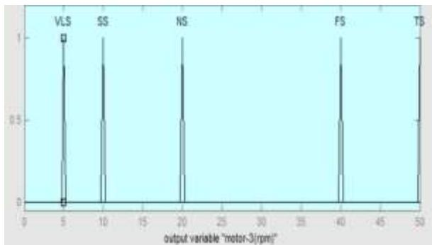
Figure 8: Membership function for motor 3 (rpm)
