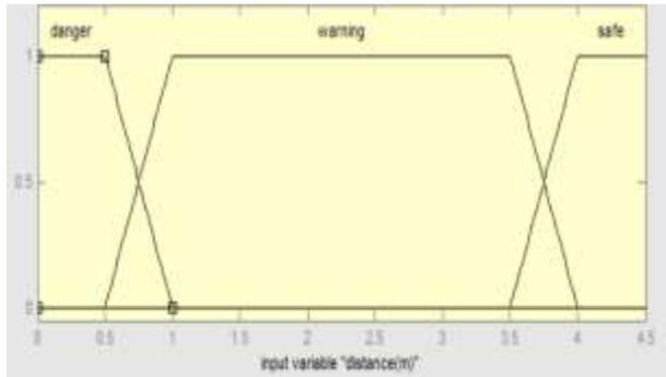
Figure 4: Membership function for distance (m)
