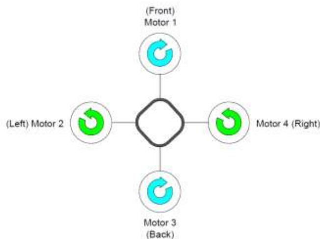
Figure 3: Quadrotor orientation
