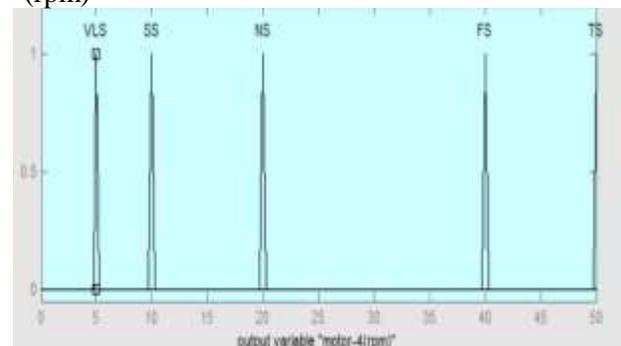
Figure 9: Membership function for motor 4 (rpm)
