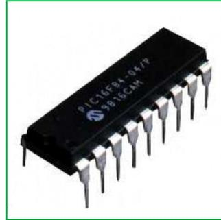
Figure 8: PIC16F84A Microcontroller
