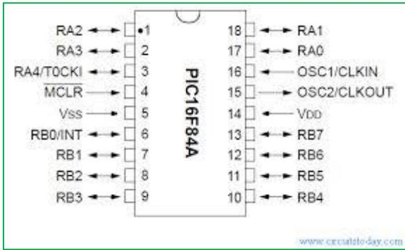
Figure 9: PIC16F84A Microcontroller PIN configuration
