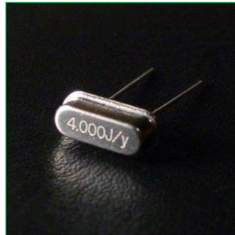
Figure 10: 4MHz Crystal Oscillator
