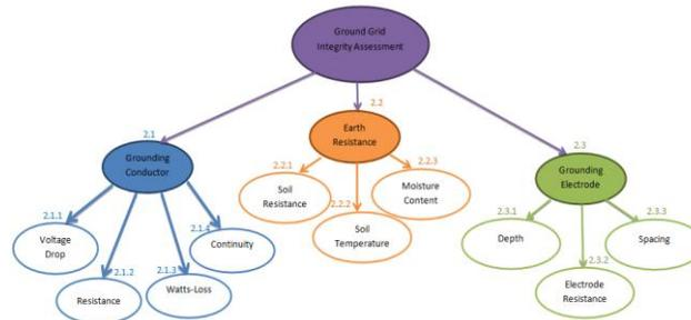
**Figure 2.2:** Precedence for the simulation of the assessment for the integrity of the grounding system
