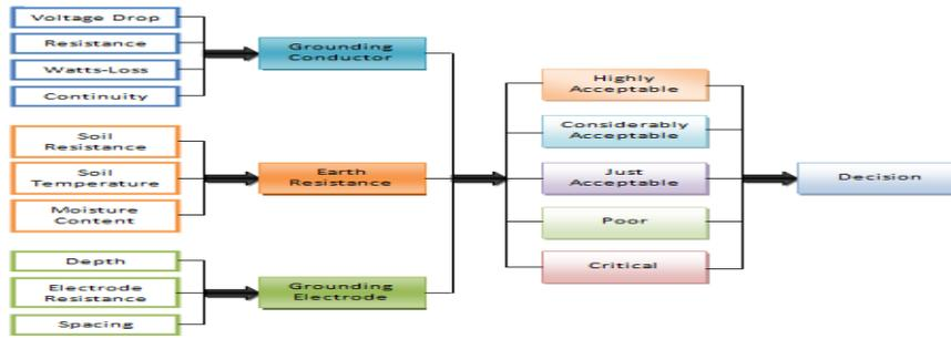
**Figure 2.1:** Hierarchical Structure for the simulation of the integrity of the grounding system.
