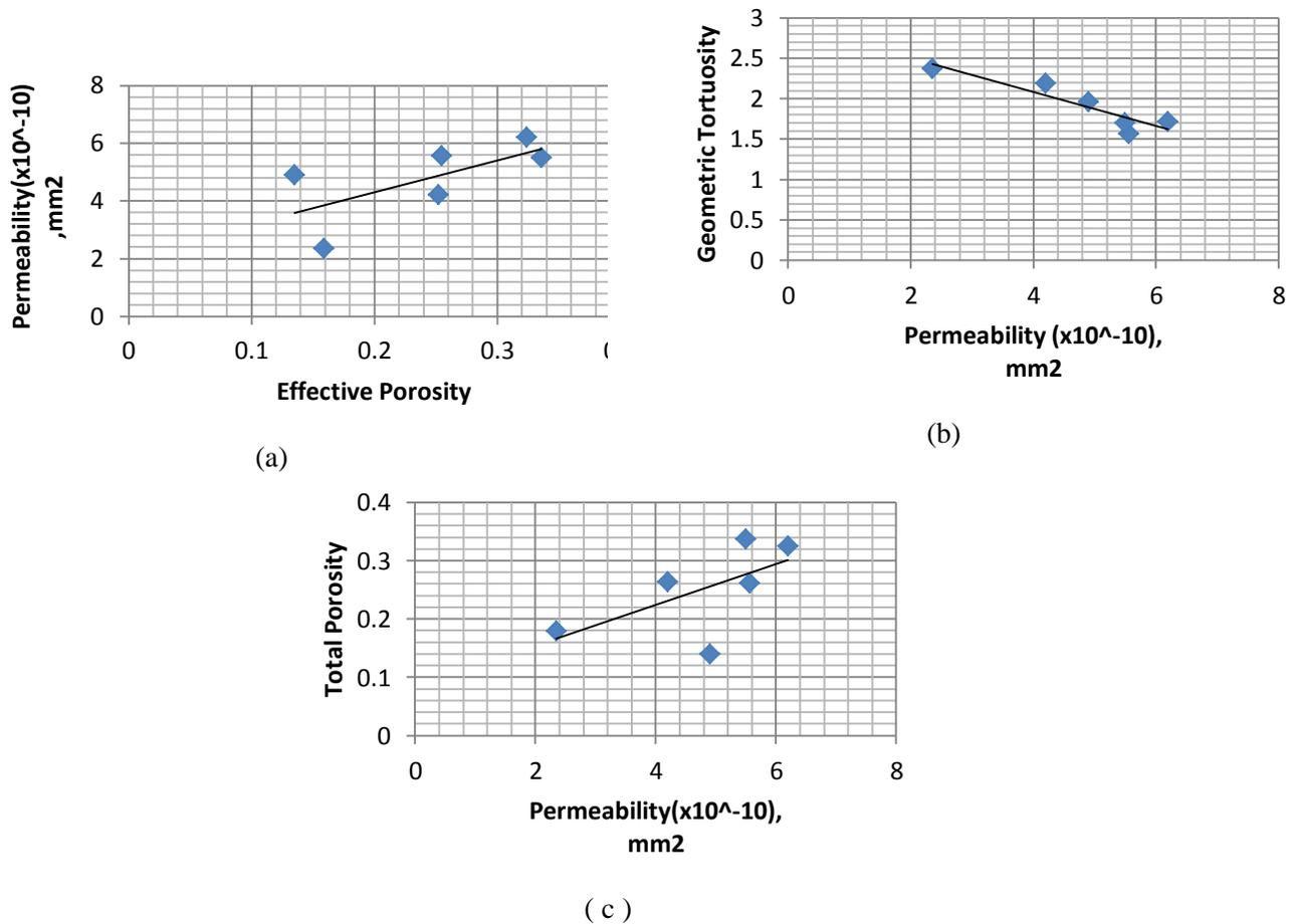
Figure 2.0 Fluid flow characterization of microstructure of pervious concrete
