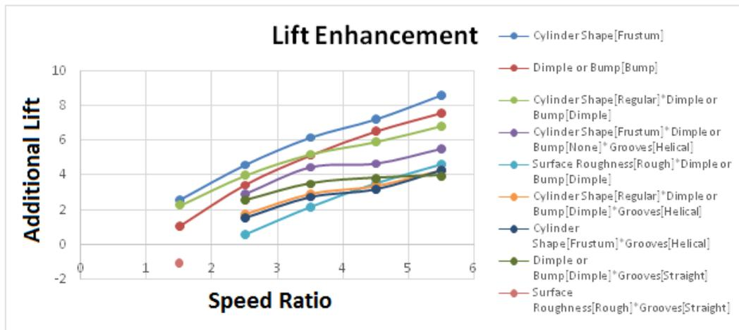
Figure 3: Estimate of additional lift provided by significant modifications
