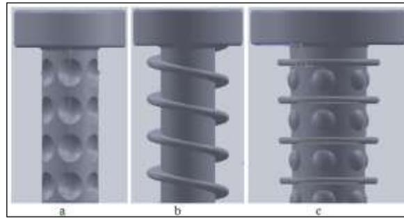
Figure 2: Some of the design geometries (a) regular-dimple, (b) regular-helical grooves, (c) frustum-bump-straight grooves. Note: Screenshots are made in different scaling.
