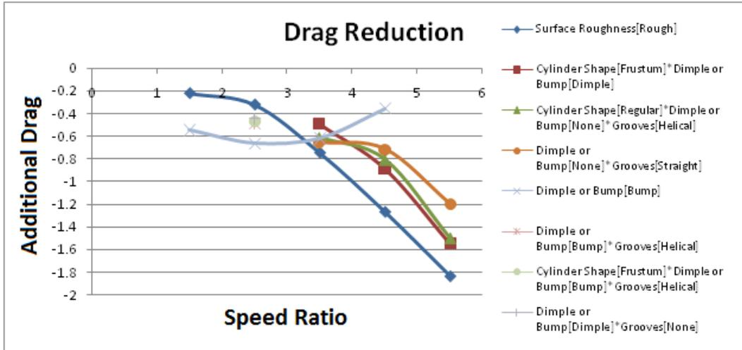
Figure 4: Estimate of additional drag provided by significant modifications
