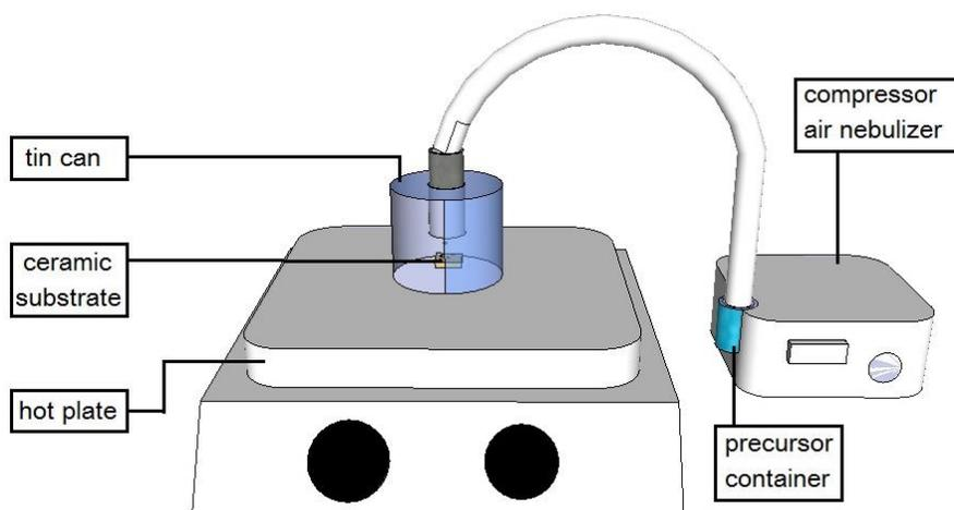
Figure 1: Schematic of Modified Spray Pyrolysis Setup using a Nebulizer
