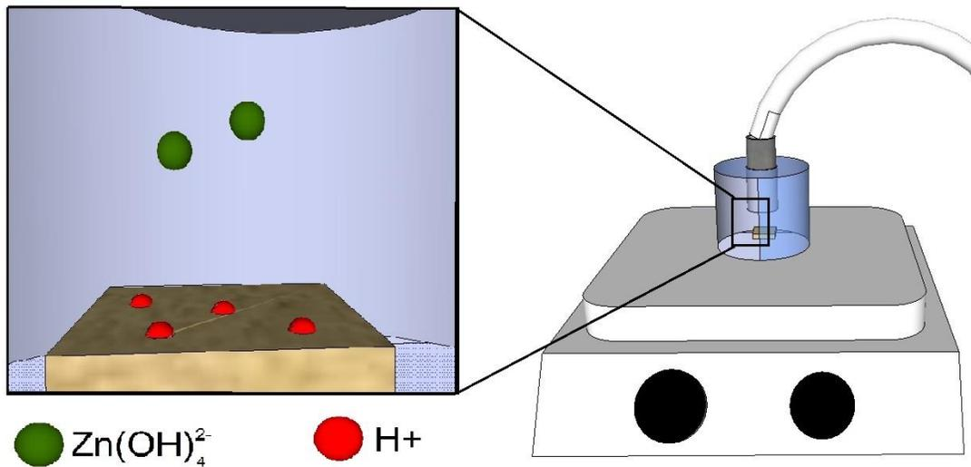
Figure 2: Proposed Deposition of ZnO via Attraction of  $Zn(OH)_4^{2-}$  droplets to the  $H^+$  seeding layer
