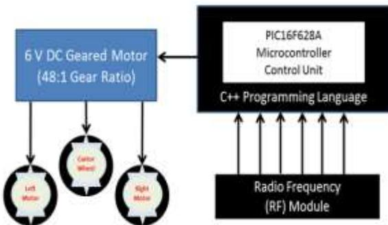
Figure 3.1: Hardware System Block Diagram
