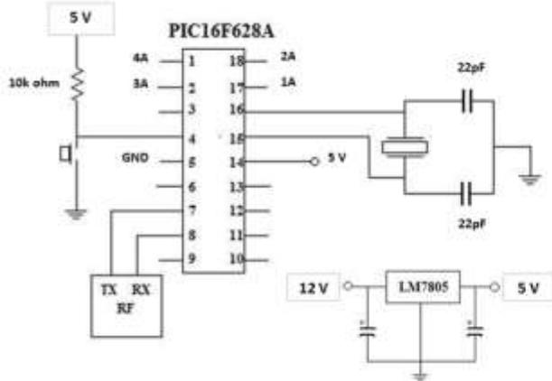
Figure 5.1: Schematic diagram of data transmission of the mobile robot
