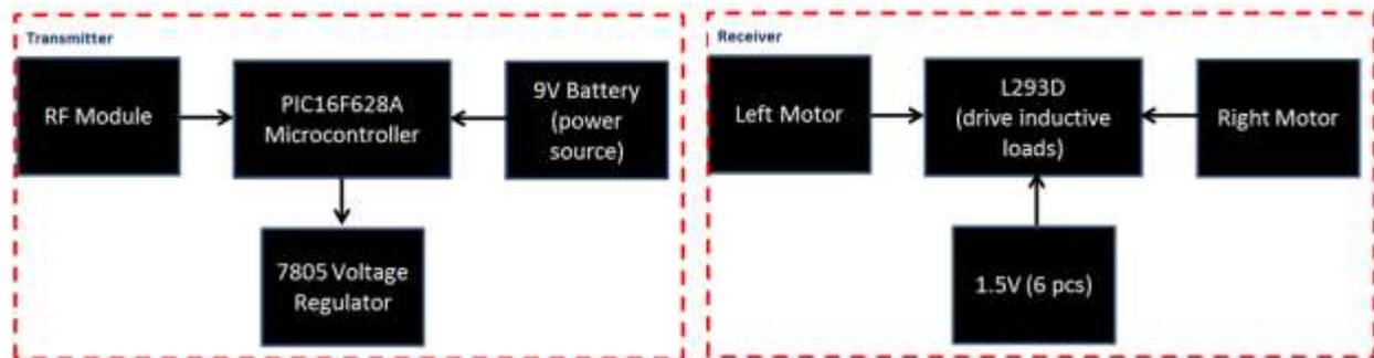
Figure 2.1: System Configuration for Mobile Robot
